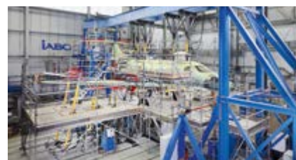
Pilatus PC-24 Full Scale Static Test (FSST)
